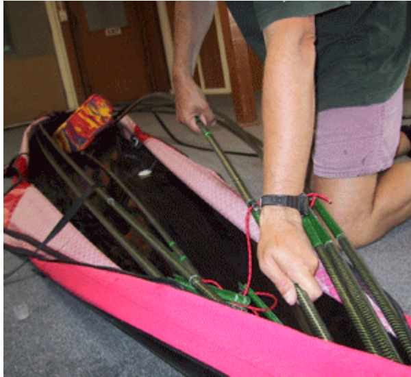
Figure 9. Inserting the green rod. Note the red, yellow and blue rods with the clips already in place, and that the seat is positioned well forwards to allow the green rods to bend and separate as the expansion clips are inserted.
