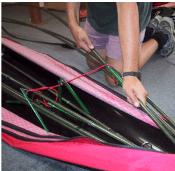
Figure 8. Inserting the clip in the blue rod. Note that the blue rod is above the yellow and red rods. This makes it easier to work on and the rods can be put back in their correct position (blue below red and yellow) once all the expansion clips are in place.
