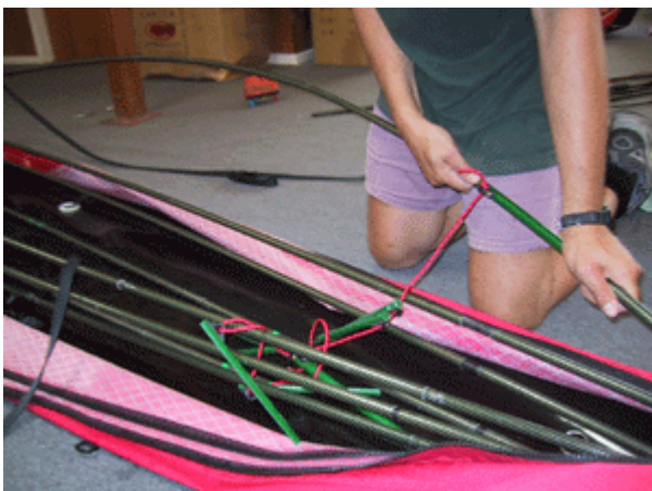
Figure 3, showing the correct positioning of the first expansion clip with the eyelet at the bow end and the remaining expansion clips on the far side of the rod.
